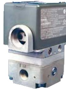
Type 1001 IP and EP Transducers from Marsh Bellofram are a patented family of electro-pneumatic instruments, used to reduce a supply pressure to a regulated output pressure which is directly proportional to a two-wire current or three-wire voltage input. This design incorporates closed loop sensing of the output pressure to achieve a typical accuracy of 0.1% and vibration stability.
