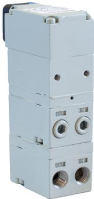
The Marsh Bellofram Type 1500 electro-pneumatic transducer converts an electrical signal to a proportional pressure output. It provides low-cost precision electro-pneumatic control to actuators, valves, positioners, final control elements and high-flow controls. Occupying a small overall footprint, Type 1500's compact size and accessibility to ports and adjustments allow the unit to be installed in space-constrained locations or in a manifold for multi-device control.
