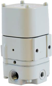
Type 1000 IP and EP Transducers are electro-pneumatic transducers that reduce a supply pressure to a regulated output pressure directly proportional to an electrical input signal. The Type 1000 accepts a wide range of supply pressures, ranging from a minimum of 3 PSIG (0.2 BAR) above the maximum output up to 100 PSIG (6.9 BAR). An integral pneumatic volume booster provides high flow capacity (up to 12 SCFM/339 slpm).
