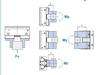
L: Distance to the point at which the load is applied (mm)
