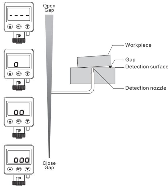
⊙ Workpiece in correct position
