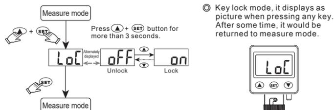
⊙ Key lock mode, it displays as picture when pressing any key. After some time, it would be returned to measure mode.
