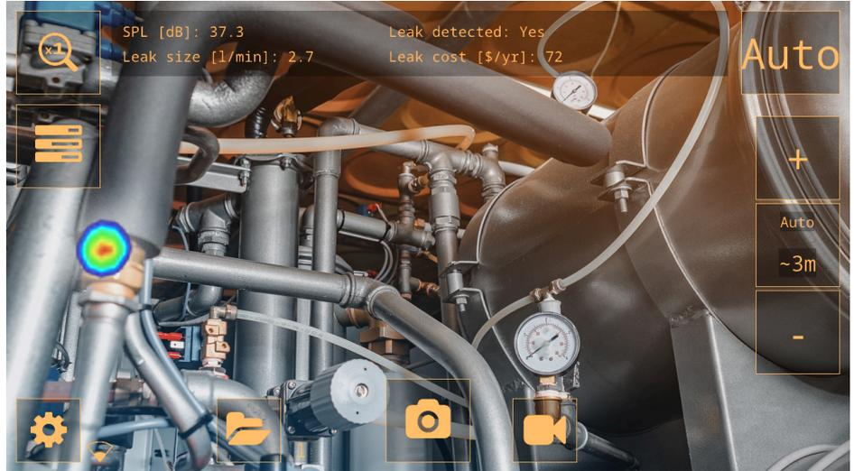
The camera can detect all kinds of pressurized gas leaks and vacuum leaks, by analyzing the sound emitted by the leak. In addition to compressed air leaks, the camera is able to detect leaks of various industrial gases.
