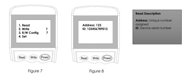
3. Press "Exit" key to go back Main Menu. Press "Power" key to switch off the programmer.
