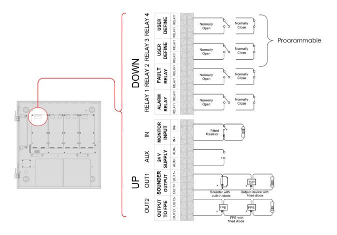
Figure 8: Input/output Wiring Details
