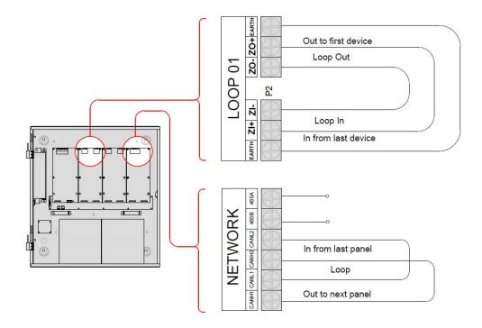
Figure 9: Loop and Network Wiring Details
