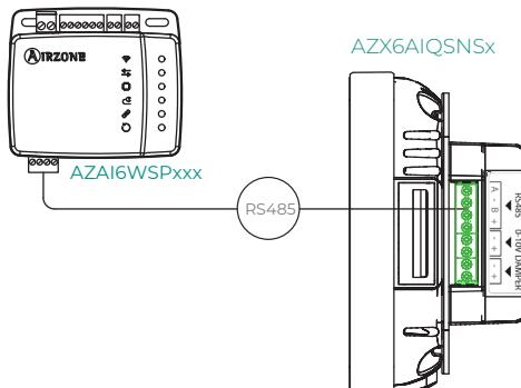
Device for the control and monitoring of indoor air quality in a zone.
