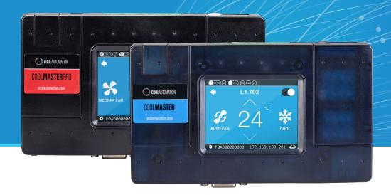
The CoolMaster product line allows home automation specialists, building automation integrators, facilities managers and HVAC professionals to integrate, control, monitor, service and manage any VRF or VRV HVAC system through a single device. The devices are Plug & Play and do not require prior technical HVAC knowledge. Simply unbox the device, ensure it is configured to the right HVAC brand using the built-in display, connect it as indicated, and... that's it!
