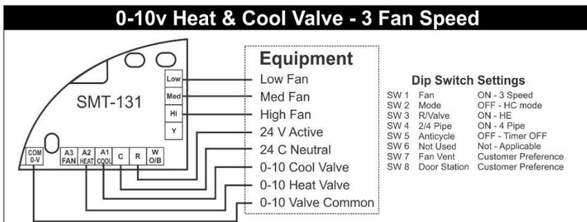
Note - When the SMT-131 calls heating or cooling the SMT-131 will drive both the relays and the 0-10V outputs simultaneously. This way the SMT-131 can call a circulating water pump via the relays as it controls room temperature with valves if needed.
