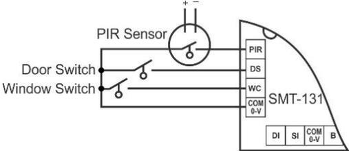
There are two types of occupancy detection modes provided by the SMT-131, see latched occupancy detection on page 11 or PIR only occupancy detection on page 12 of this manual.
