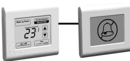
Connection between the SMT-131 and the hotel door station is cable fitted with RJ12 plugs. Cables can be provided at additional cost at up to 15 metres maximum. Alternatively, custom cables can be produced. They are direct wired (not cross over).
