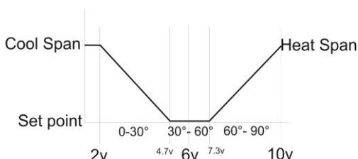
**Note** When using “Belimo”™ mode, both the A1 “cool” and the A2 “Heat” 0-10 output are used. Both will provide the same output to the valve. (The A3 “fan” output will remain unchanged and can be used to control a DC fan or other devices).
