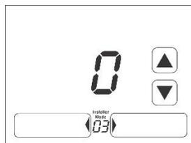
The current menu option is shown between the left and right buttons. The example to the right shows option 3, select deg C (option 0) or F display (option 1).
