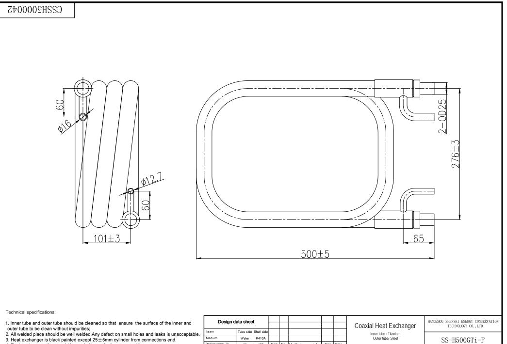
4. Each end connection should be sealed by a plastic cap or welding.
