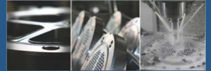
FOUR-AXIS MACHINING CENTER TUBE PLATE PROCESSING, EQUIPMENT FLANGE PROCESSING AND SEALING SURFACE PROCESSING WITH HIGH PRECISION, 4 GROOVES IN TUBE SHEET PROCESSING
