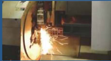
LASER TUBE CUTTING PROCESS SHELL CUTTING AND PROCESSING, INLET AND OUTLET PIPE PROCESSING
