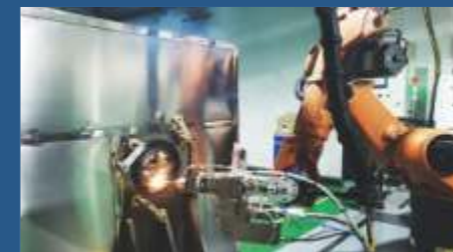
FLUORINE SIDE HEAD LASER WELDING LARGE PENETRATION DEPTH, HIGH PENETRATION RATE, SMALL HEAT-AFFECTED ZONE, EXTREMELY FAST COOLING
