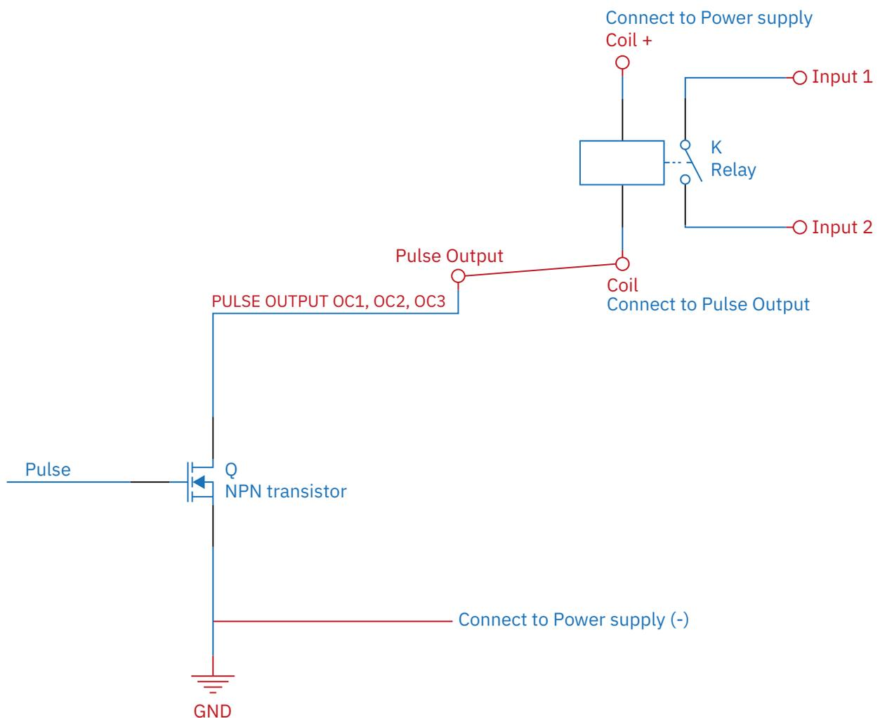
It's necessary to select an appropriate relay:
