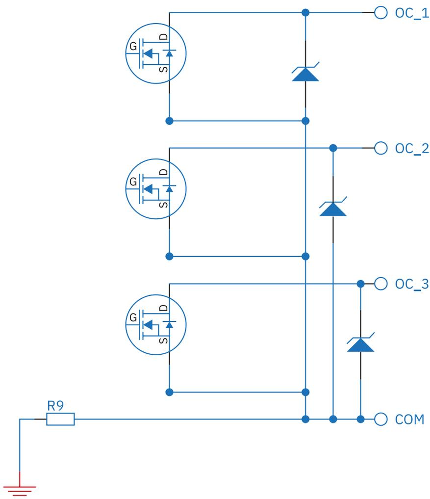
The figure shows that the OC\_1, OC\_2, OC\_3 outputs (where we'll connect the PLC input or any device that receives the pulses) are connected to an N-MOS type transistor (J1, J2, J3 in the figure). The output operation is as follow:
