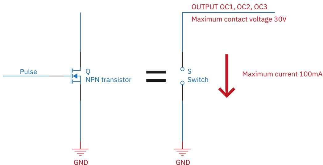
This type of output (Open Drain) is usually accepted as valid for devices such as PLCs. However, it's necessary to check that the voltage applied to the contact, by the external device, does not exceed the maximum bearable voltage. For **IWM-PL3** and **IWM-PL4** products this voltage is 30V in continuous electric current (DC).
