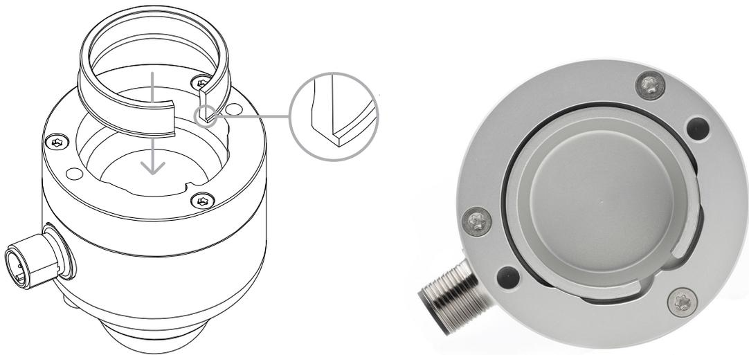
**Figure 5.4.1.1** Line drawing indicating placement of the aluminium shim and photo showing the shim properly positioned in the centre of SR05's bottom plate. Note the position of the protruding ledge when placing the shim.
