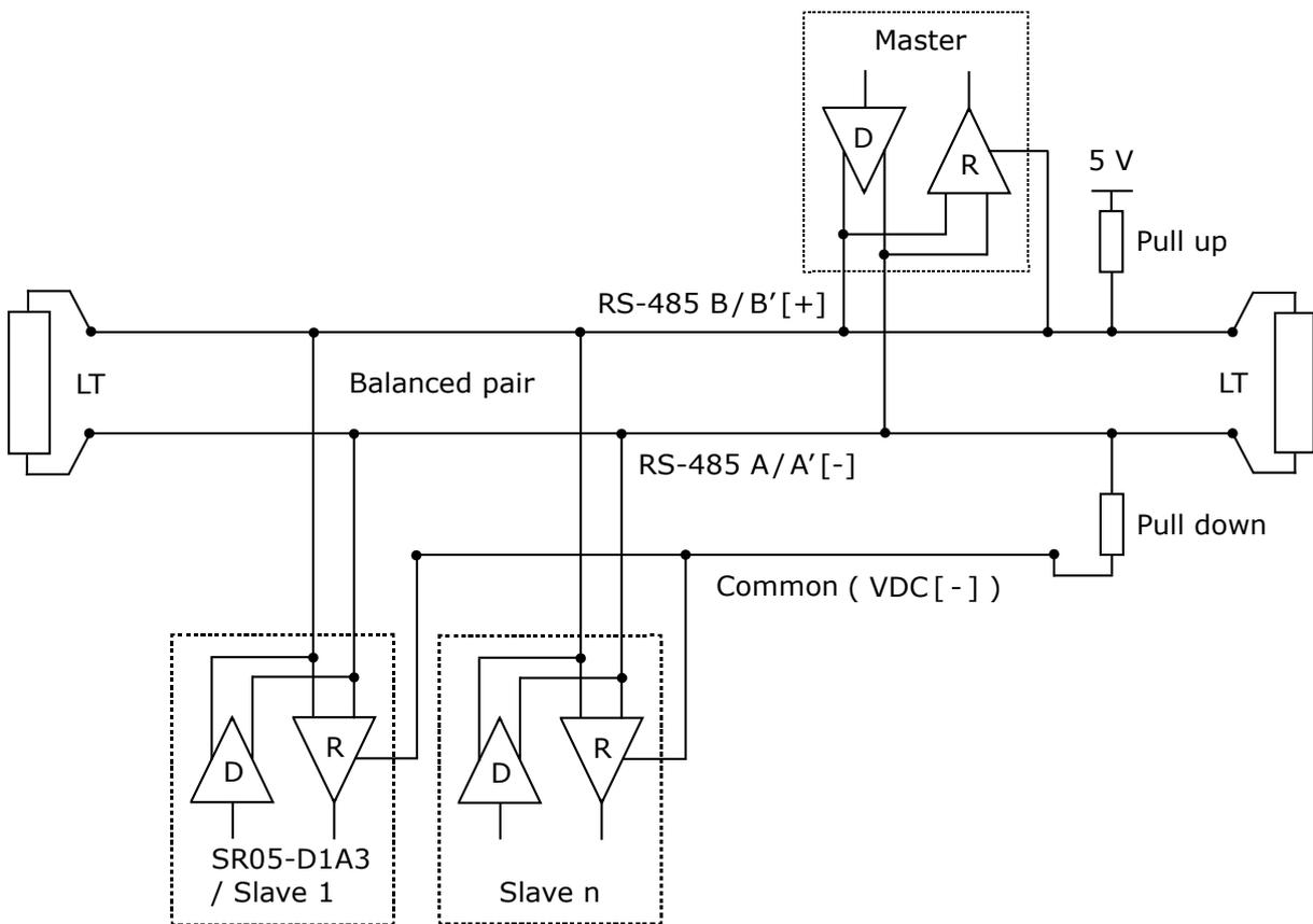
**Figure 5.10.1** Typical topology of a two-wire RS-485 network, figure adapted from: *Modbus over serial line specification and implementation guide V1.02 (www.modbus.org)*. The power supply is not shown in this figure.
