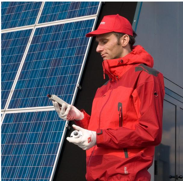
**Figure 2** Pyranometer in use with LI19 read-out unit.
