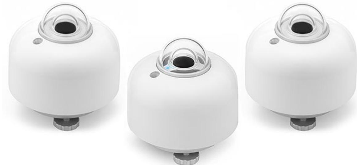
**Figure 0.1** Industrial pyranometer models SR300-D1, SR200-D1 and SR100-D1. In front the leading Class A model SR300-D1, with heating, tilt sensor and the blue status LED. Left and right the non-heated Class A model SR200-D1 and Class B model SR100-D1.
