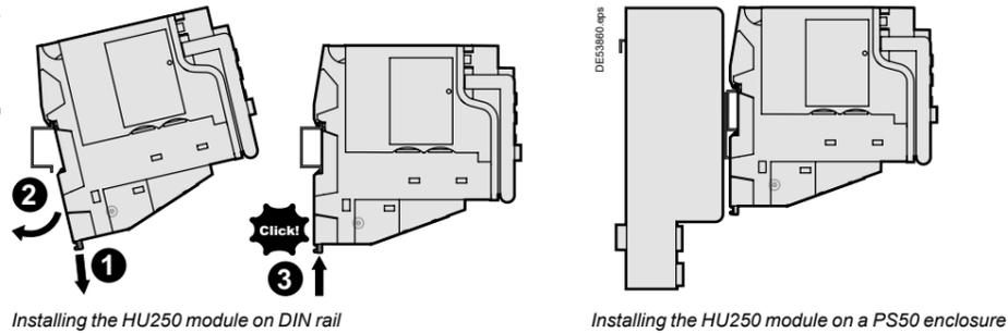
Installing the HU250 module on DIN rail
