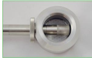
5. Place the cover onto the calibration chamber and close it tightly. The hygrometer is now ready for calibration or adjustment.
