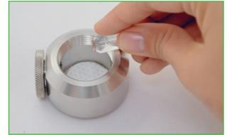
4. Insert the probe into the calibration chamber till it reaches the opposite side. The sensing head (tip of the probe) shall not come in contact with the salt solution.
