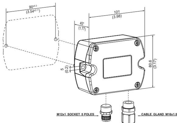
\*The polycarbonate enclosure without display: 46 mm (1.81").
