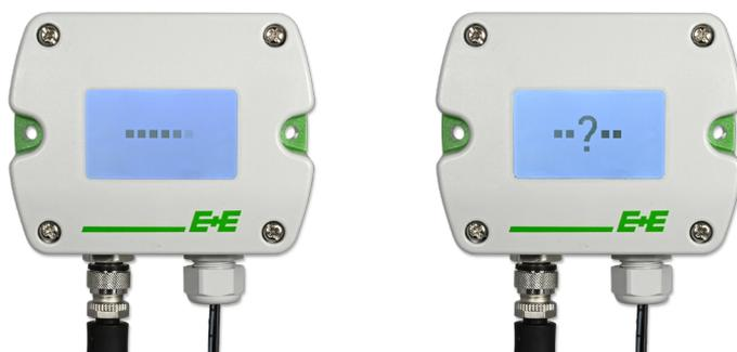
Fig. 3 Display during RS485 interface scan
