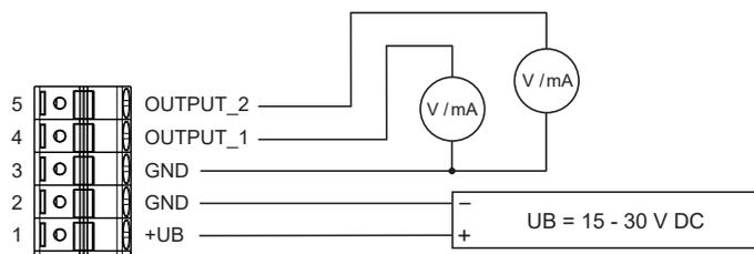
Fig. 1 Voltage supply and outputs
