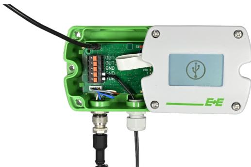
Fig. 5 Sigma 05 with USB connection active only
