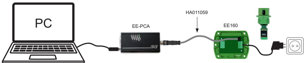
Fig. 13 EE160 configuration analogue output using EE-PCA kit
