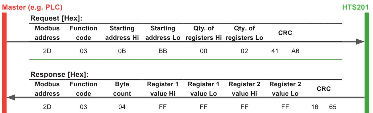
Fig. 4 Query of an unconfigured custom Modbus map
