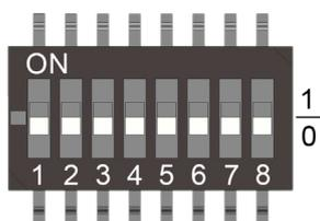
All DIP switches at position 0 → address has to be set via PCS10
