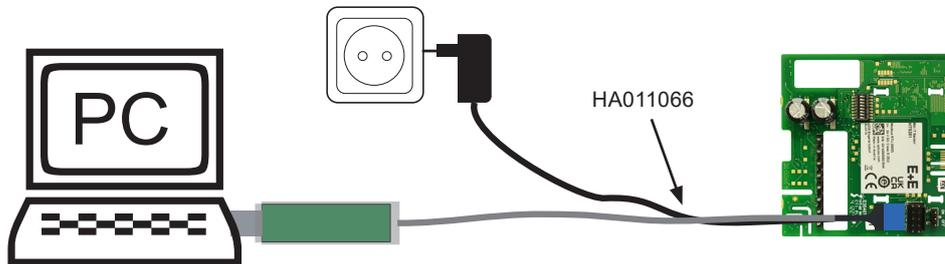
Fig. 1 HTS201 connected to a PC running PCS10
