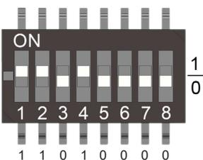
Modbus address setting via DIP switch:
