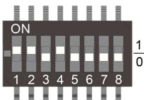
**Modbus** (slave device): Setting the DIP switches to any other address than 0, overrules the Modbus address set via PCS10 (permitted values: 1...247).
