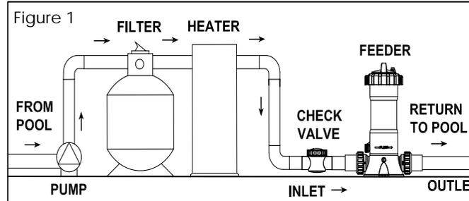
At the inlet pipe to the feeder, a positive seal corrosion-resistant check valve should be installed to reduce backflow of chlorine gas when the system is turned off. It is recommended that if the feeder is installed below the waterline, a check valve is needed to prevent water backflow when opening the unit.
