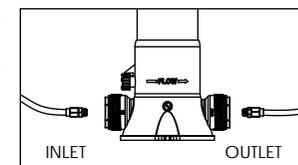
**Note:** After installation start up the system to perform leakage check, re-tighten if required. The feeder can be fixed onto the installation surface by tapping screws and securing holes in its base.
