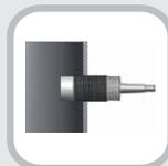
For the level control of liquids or bulk materials the best sensors to deploy are Non-Flush format with the active surface of the sensor in direct contact with the media to be detected
