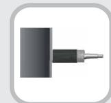
Flush format sensors have the option to control product levels through a non-metal container wall. The wall thickness should not exceed 4mm at the sensing location
