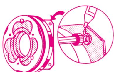
4. After adjusting the gap (dimension g) between the frictional faces with the attached shim, install the system. Refer to Table 1.
