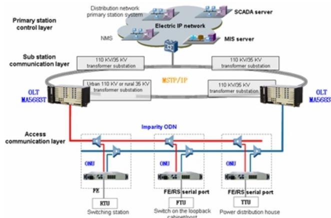
Figure 1-2 Network topology application for automatic power distribution in the electric power industry
