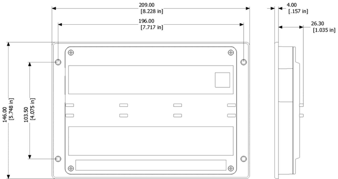
Mounting holes suitable for 4 x 4mm screws
