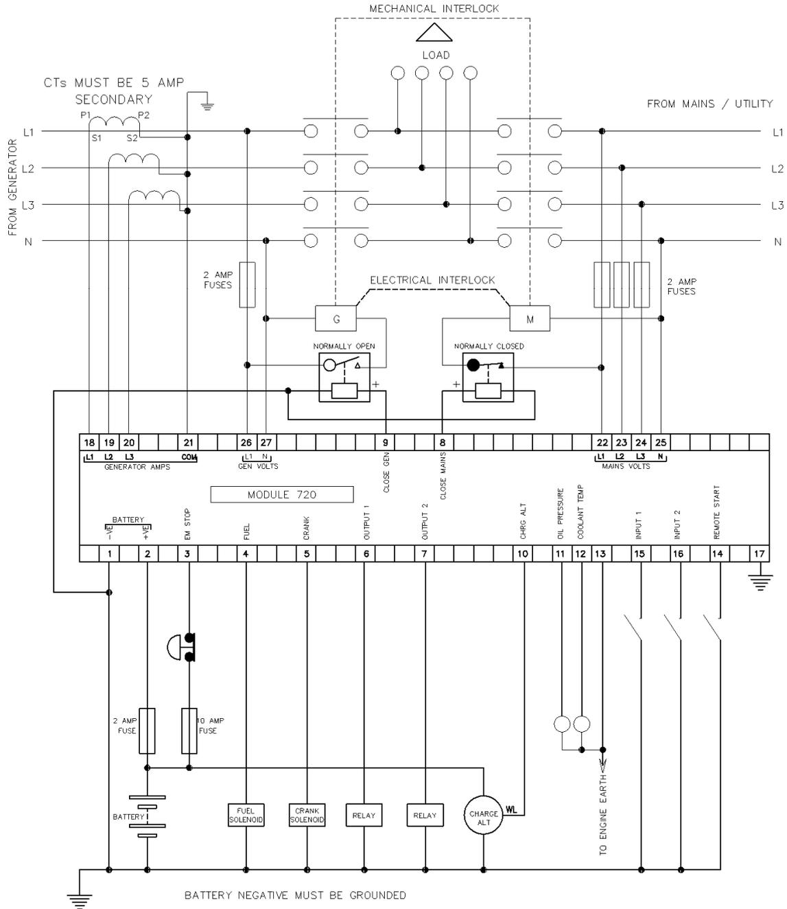
SCREW TERMINALS TIGHTENING TORQUE = 0.8Nm (7lb-in)
