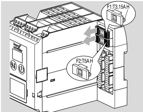
5 Check fine-wire fuse F1 or F2 for correct functioning.
