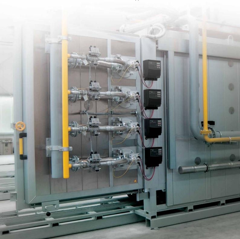
Honeywell's next-generation Kromschröder® BCU 4 Series burner controls – encompassing BCU 460, 465 and 480 models – feature modular, all-in-one designs that can be mounted close to industrial burners to facilitate system integration, offering good value.
