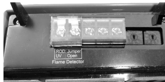
ULT Model (bus connector and address switches)
