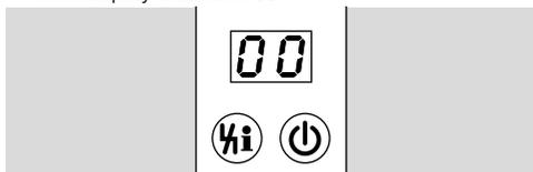
→ The IFD retains its switch position when the voltage is removed from terminal 1.
