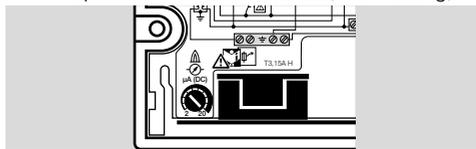
→ The fuse only protects the ignition output! After a short-circuit on the valve output, an internal fuse in the unit trips, which cannot be changed. Return the unit to the manufacturer for inspection.
