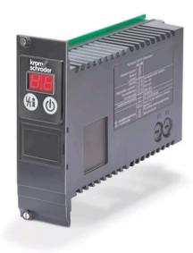
For controlling, igniting and monitoring impulse-controlled, modulating or stage-controlled gas burners, for continuous operation with ionization control, for intermittent operation with UV control (with UV sensors of type UVS) or as a variant for continuous operation with UV control (with UV sensor UVD 1).
