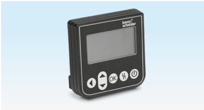
The OCU is an external operator-control unit which can be connected to a control unit of the FCU 500/BCU 500 series. The external operator-control unit OCU is installed in the door of a control cabinet. Thus, the control cabinet does not need to be opened to read out process values, statistics, flame signal intensities or parameter values, to change settings on the OCU or to control or adjust connected valves in Manual mode.
