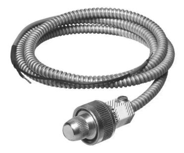
The C7915 Flame Sensor includes a lead sulfide photocell that is sensitive to the infrared radiation emitted by the combustion of fuels such as natural gas, oil, and coal.
