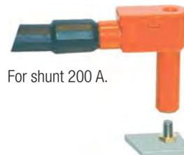
Clamp with tapped revolving rod end M8, 200 A shunt. To be used with an insulating six-sided male hex key 5 mm.
