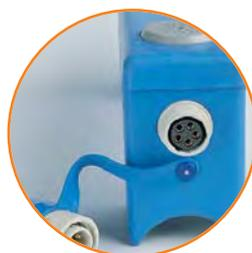
The phase is identified with an amperemetric clamp connected to the receiver and positioned around the phase to be identified. When the clamp detects pulses drawn by the modulator, the receiver emits a light signal, confirmed by a beep after three seconds.
