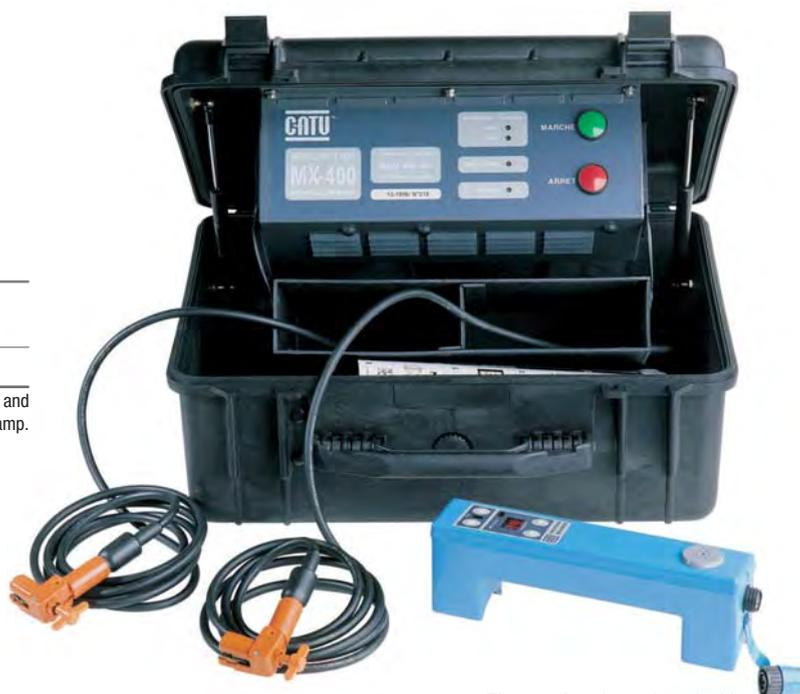
**H07RNF power cables.** (6 mm<sup>2</sup> and 3 m length). The connection is made between phases for identifying the cable or between phase and neutral for identifying a phase. After connection, the device is immediately live, as indicated by two 230 and 400 Volts lights.
