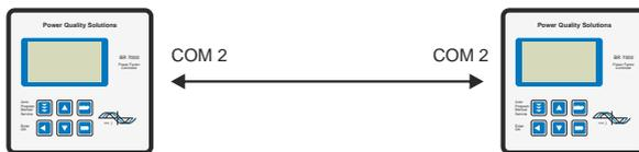
The operation mode coupling operation (parallel operation resp. master-slave-operation) is selected in the program-mode under 23 EXTERNAL INPUT.
