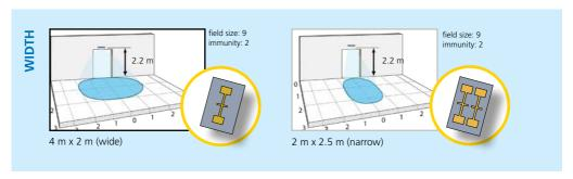
The size of the detection field varies according to the mounting height of the sensor.
