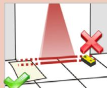
Always verify the actual detection field width with a piece of paper and not the Spotfinder, which detects the whole emitted field.
