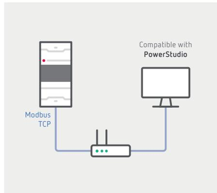
*Connect the analyzer to the local network and start measuring.*
