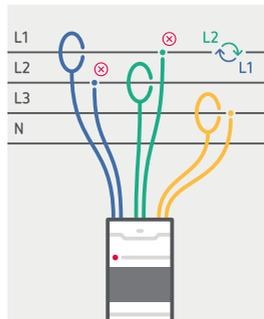
Error installing current sensors
