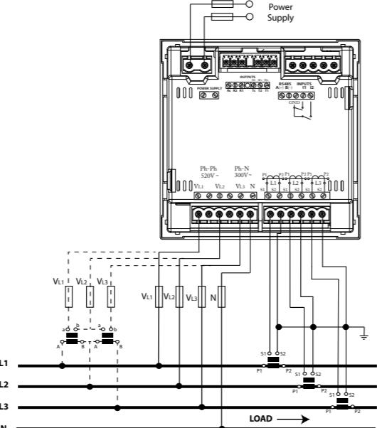
Red trifásica a 3 hilos / 3-wire three-phase network
