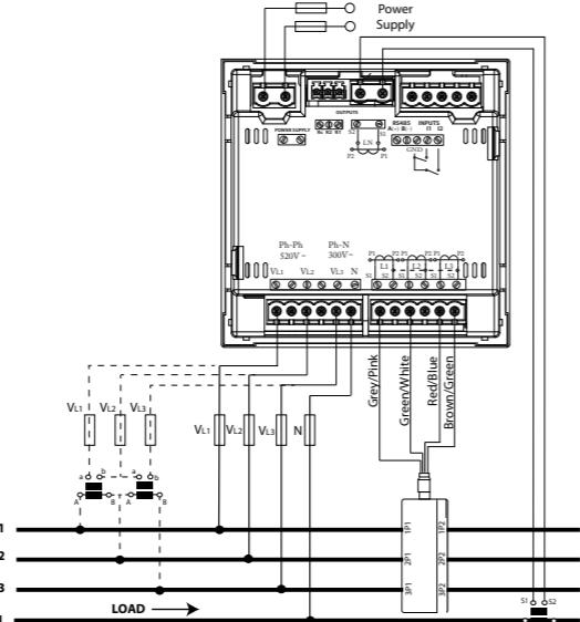
Red trifásica a 3 hilos / 3-wire three-phase network
