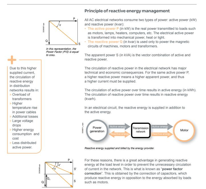
The result is a reduced apparent power, and an improved power factor P/S' as illustrated in the diagram opposite.
