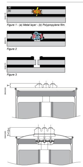
Cross-section view of a three-phase capacitor after Pressure Sensitive Device operated: bended lid and disconnected wires. **Self-healing** is a process by which the capacitor restores itself in the event of a fault in the dielectric which can happen during high overloads, voltage transients etc.
