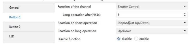
Fig. 4.6 Parameter Setting Page "Button x- Shutter control"
