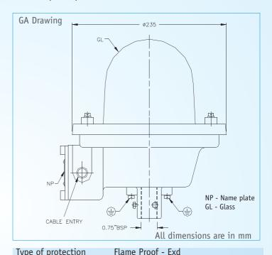
Type of protection Area Classification Zone 1 & 2 Group I, II A ,II B Gas Groups IS - IS-13346/2004 (IEC 60079-0/200) Apparatus Standard
