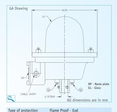
Type of protection Area Classification Zone 1 & 2 Gas Groups Group I, II A, II B IS-13346/2004 (IEC 60079-0/200) Apparatus Standard IS-2148/2004 (IEC 60079-1/2001) CMRI Certificate No. CMRI / TC / P / H 1308
