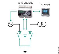
Transformer/transformer and transformer/genset applications.
