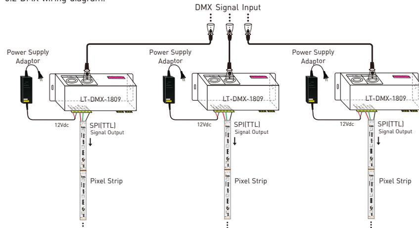
\* An amplifier is needed when more than 32 decoders are connected, signal amplification should not be more than 5 times continuously.
