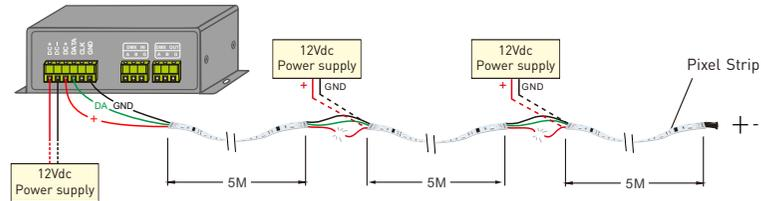
B. Special connection method - light fixtures and controller using different operating voltages.
