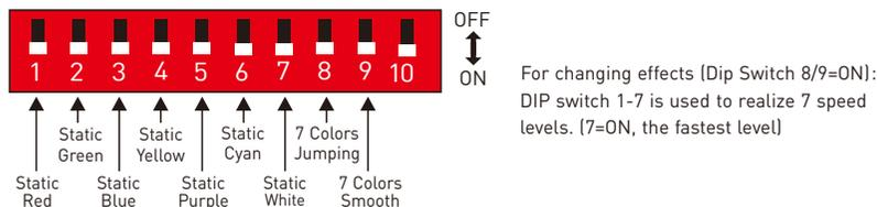
[Attn] When several dip switches are ON, subjected to the highest switch value. As the figure above shows, the effect will be 7 colors smooth at 7 speed level.
