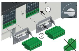
Connect the product with a cable of section of 1,5 to 2,5 mm<sup>2</sup>.
