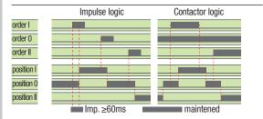
To enable control, close contact 312 with 317. To force the product to 0 position/OFF bridge the contact 313 with 317. For contactor logic bridge contact 316 with 317. To operate: close the contact corresponding to the desired position.
