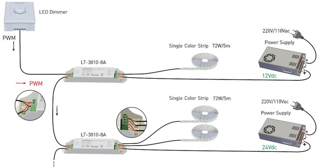
Power repeater connected to LED dimming driver:
