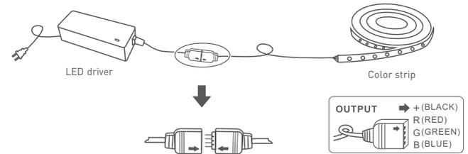
[Please connecting the LEDs in power off, and power on in correct connection.]
