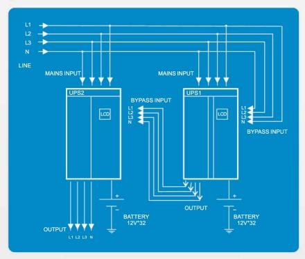
Line Connection for Y input and Y output
